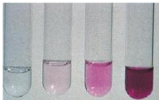
Nitrate Reduction Test Showing Negative (-) as well as Positive (+) result (Right Handed Test Tube) Respectly.
